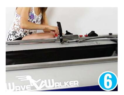
Remove the right cross bar screw & slide the rudder assembly under the cross bar.
