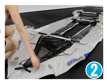
Remove the covers from the air valves and turn the air valve stems until they pop up in the "noair flow" position.
