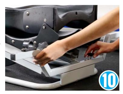
Now, lift the frame assembly and place it between the side support bars into the hull. You may have to pull the hulls apart slightly so the frame can settle between the pontoons. Press the frame assembly down firmly until the support bars rest on the side support bars.
