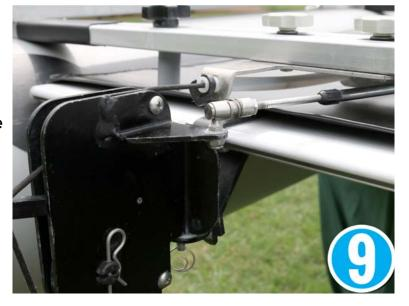
Next, attach the front and rear support bars to the drive frame assembly with the provided screws.
