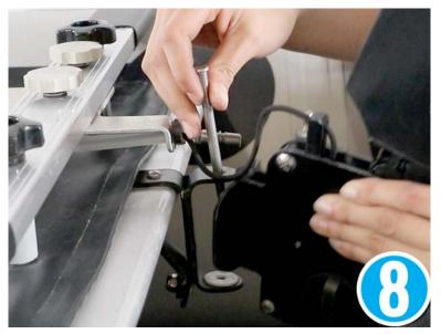
Connect the steering cable's spring-loaded end to the ball on the rudder assembly by pulling back the spring loaded sleeve, placing the end over the ball, and sliding the sleeve back into place.
