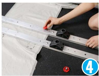
Now, place the side support bars across the top of each pontoon, with arrows pointing forward.
