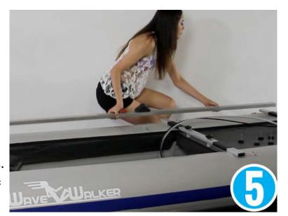
Now, place the steering assembly on the inflated hull assembly, and attach the steering handle assembly to the right side support bar with two screws.
