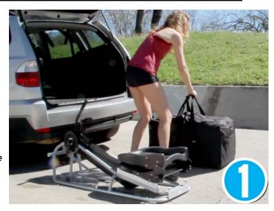
Loosen the straps on the carrying bag, opening the bag's flaps, and roll out the hull assembly, making sure it's right-side up.
