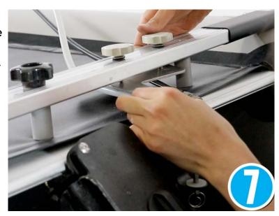
Remove the rudder pin from the rudder bracket by rotating the circular cotter pin.
